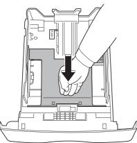
3 Setup the back side feed cassette stop by pushing the "PUSH" lever (A).
